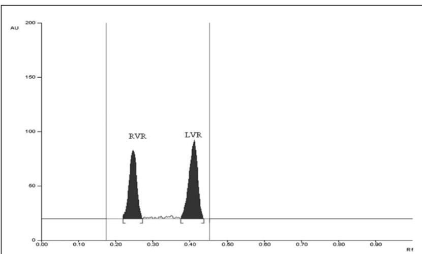
**Fig. 4:** Densitogram of Ritonavir (Peak-1(RVR): 800 ng/band,  $R_f = 0.242 \pm 0.03$ ) and Lopinavir (Peak-2 (LVR): 3200 ng/band,  $R_f = 0.413 \pm 0.02$ ) of formulation (EMLETRA) showing no interference of excipients in analysis
